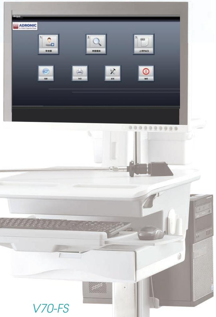
Adronic PACS Image System Station is a stander of DICOM 3.0 format, its image data picture or video that allow to upload directly to hospital PACS database in time.
